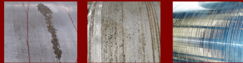
Look familiar? Typical flaking and corrosion on chrome-plated glue roll: scoring on doctor roll.
